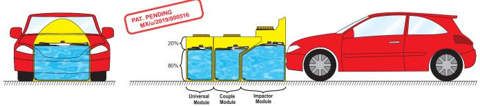
First, the flexible inner container arrangement of each module fills with water up to 80 % of the volume of the third external container, then the container must be well closed, sealed with no air inside, and fold the empty part inside the external container.
