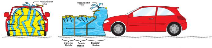
Depending on the kinetic energy, the external container can be destroyed and the safety valves open letting the water flow by oriented holes and in a controlled way, while they still had been absorbing the speed and the mass momentum of the vehicle.
