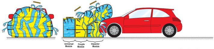
The impact can rip the container but the arrangement continues damping the vehicle, the container takes the shape of the front of the car increasing the contact area and therefore, the cushioning effect. This engineered solution saves lives, and diminishes damage extension.
