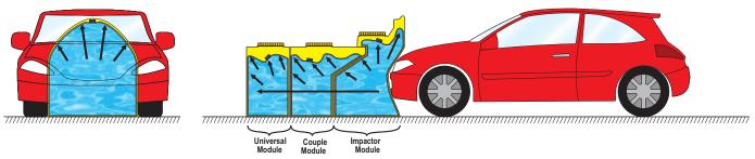
When the first module receives the impact, it deforms and passes the shock pressure to the next containers forcing water movement to the empty room.
