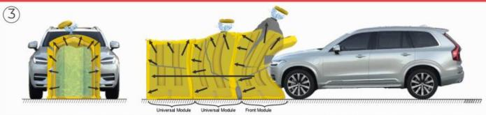
If the pressure exerted during the impact or collision is too high, the relief pressure valve is opened and allows the water to come out in a controlled manner, so part of the pressure exerted on the water is released and the contact time between the vehicle and the triple container system is longer.
