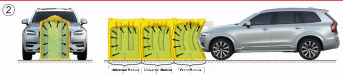
From the moment the vehicle contacts the first module, the impact attenuation process is activated. The outer container deforms and may rupture upon impact. Meanwhile, the inner flexible containers are compressed, causing the water inside to shift. This allows the containers to conform to the shape of the vehicle's front end, effectively wrapping around it and absorbing the collision energy.
