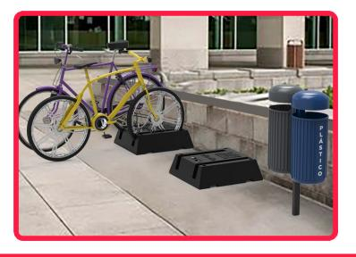
Installation Mark the four boreholes of each base. Ultrafix hex-head screw Bore into the holes with the help 21v Ø 3/8" × 5.85 in. of a drill and a 3/4" concrete drill bit to a depth of 7". Flat washer. Place the anchors on the boreholes. Leg. Put the dual bike rack. Insert the screws and the Extralarge anchor 3/8" flat washers. Ø 0.70 in. x 5.26 in. Perfectly tighten the four screws with a 9/16" socket wrench. The installation is ready. Borehole.
