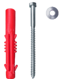
Anclaje en concreto Taquete "Extralarge" (3/4" x 14 cm) Tornillo "Ultrafix" (3/8" x 15 cm)
