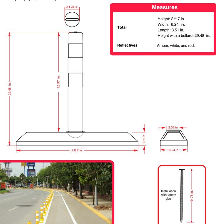
Installation on asphalt Steel nail (1/2" × 9.75 in.)
