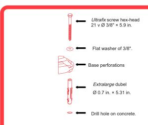
Mark the three holes where the posts are going to be and with the help of a drill with a ¾" concrete drill bit bore into a depth of 7" and put the *Extralarge* dubels on each hole. Assemble the **Folding Post** with a screw and a 3/8" flat washer. You can do this with the help of a 9/16 socket attached to a T-Handle socket wrench. Pierce the post and spin the screw to the right until it is tight enough. Like this, the installation is completed.
