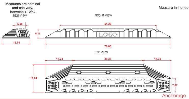
Floor anchorage with 7 nails 1/2" x 10" and epoxic glue
