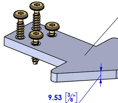
The assembly of the speed hump without anchors through steel plates with the shape of an arrow of 9.53 mm (3/8 ") and 4 lag screws.
