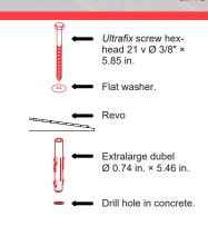
The Revo will act as a template. Mark all the holes with a drill and a 3/4" drill bit. Then, bore into the marked area at a depth of 7". Put the dubels in the holes, assemble the speed hump, insert the screws and flat washers of 3/8" and perfectly tighten them with a 9/16" socket.
